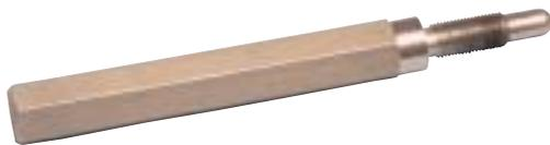
A piston stop threads into the spark plug hole to provide a consistent point for halting the piston's trip up the cylinder. Using some simple averaging, you determine the exact location of TDC.
