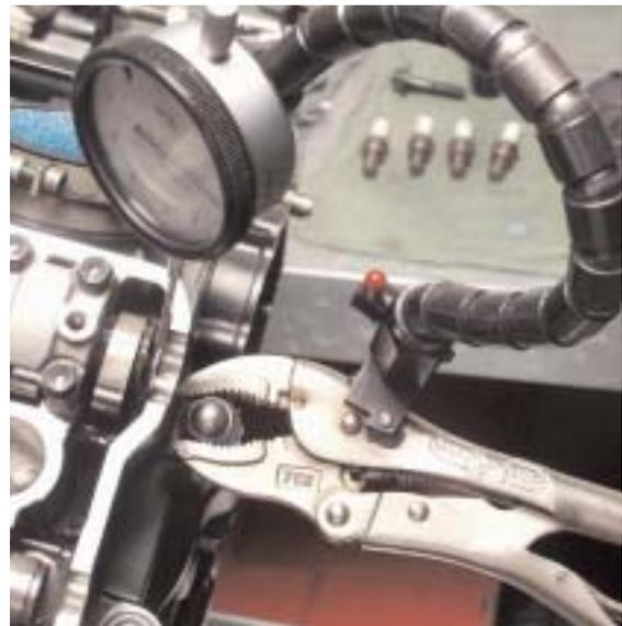
The dial indicator needs to be solidly mounted to the engine. Make sure that the plunger moves parallel to the valve and has enough range to track the valve through its maximum extension.
