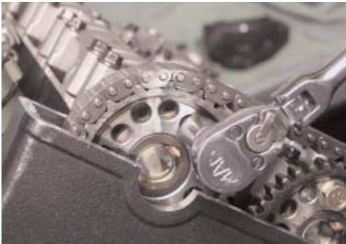
To alter the cam lobe's center, you need to loosen the sprocket bolts and move the crankshaft slightly.
